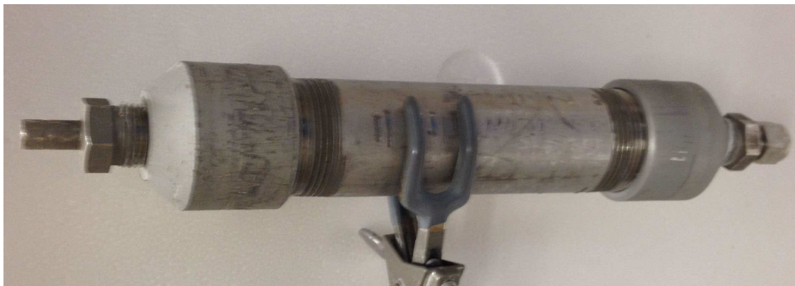
Figure 2.1.: Photograph of Passive Surface Water Flux Meter.
