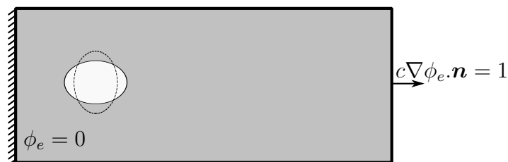
Figure 4.10. Loading conditions for the kidney formation (Fig. 4.11) and void splitting examples (Fig. 4.12).
