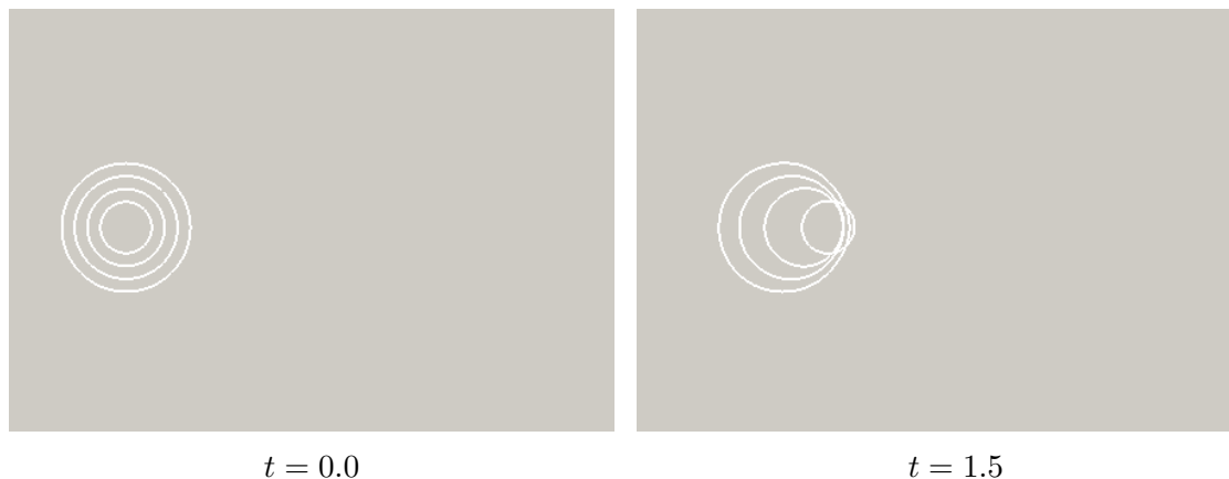
(a) Initial and final location of voids of various sizes, under constant electrical potential gradient.
