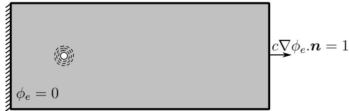
Figure 4.6. Boundary conditions for the validation examples.
