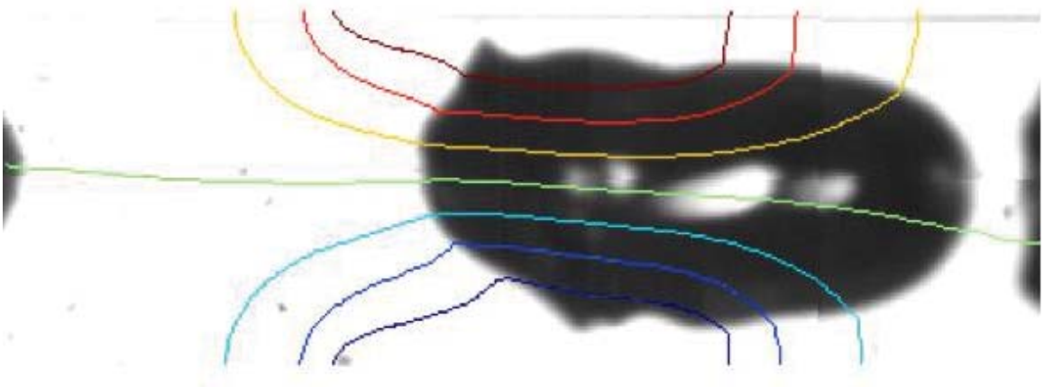
Figure 4.6. Constant potential lines superposed on an image of a slug bubble used in a simulation. The void fraction for this video is 0.33 and the simulated impedance is 0.41.
