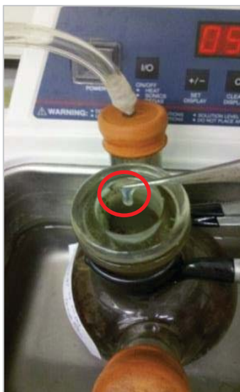
Figure 3.5. BNC pellicle before impregnation of IONP (red circle). Pellicle is clear and slimy before the reaction.
