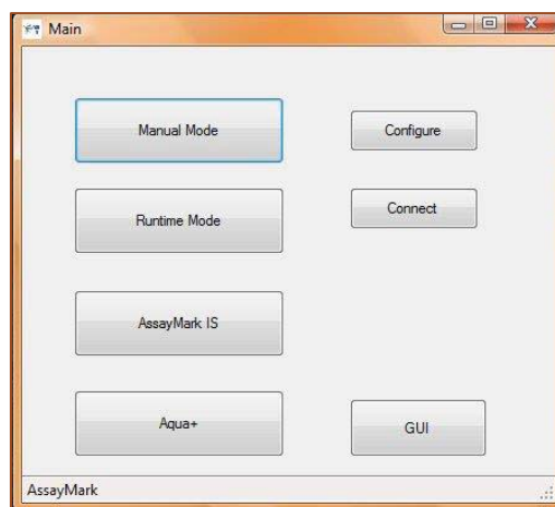
Figure 5.5. Assay Mark opening GUI. “Connect” button is used to connect the controller box to the laptop. The “Manual Mode” button is selected for normal operations.
