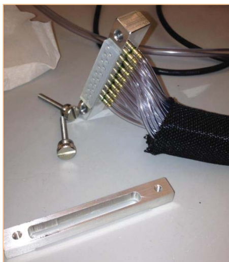
Figure 5.4. Close-up of manifold connected to microfluidic lines (tubing). These lines are responsible for pressure and vacuum going into the bioMEMS chip.
