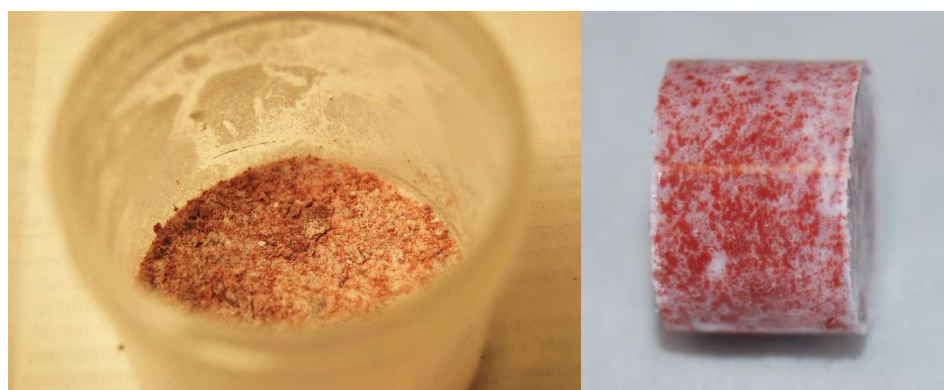
Figure 2.11 A mixture of 80% EDBB/20% RTV after being mixed on the Resodyn (a) and then pressed in the carver press (b).
