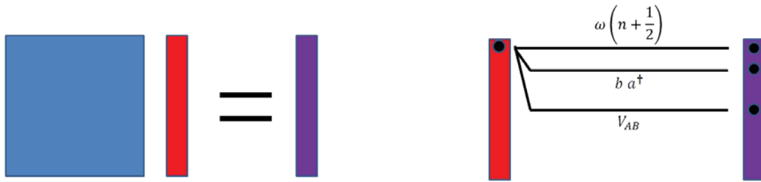
Figure 4.1. Traditional matrix multiplication, left, requires the entire Hamiltonian to be constructed to find the red product vector. The matrix/vector product algorithm in EVspectrum, pictured right, uses the operator form of the Hamiltonian to compute the matrix vector product.
