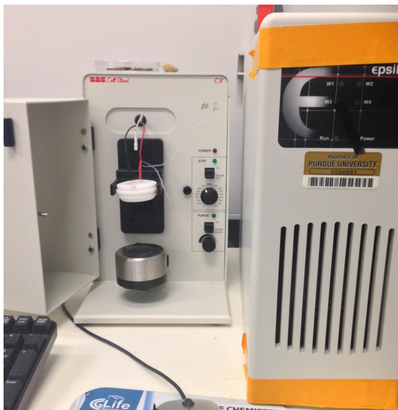
Figure 3.14 Cell stand (left) and EC epsilon potentiostat (right) for open circuit potential measurement of calcium concentration.
