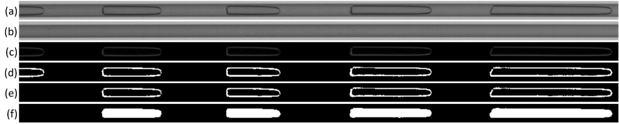
Fig. 3. Selected frame showing the (a) original image, (b) background image, (c) gray-scale image after background subtraction, (d) binary image after thresholding, (e) binary image after removing partial bubble interfaces, and (f) final binary image with vapor bubbles filled in white.
