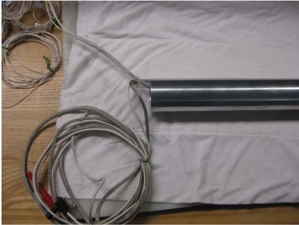
Fig. 6.17. Picture of the leads to the glow perturber and the Kulite pressure transducers coming out the back of the 30-degree cone-ogive-cylinder model.
