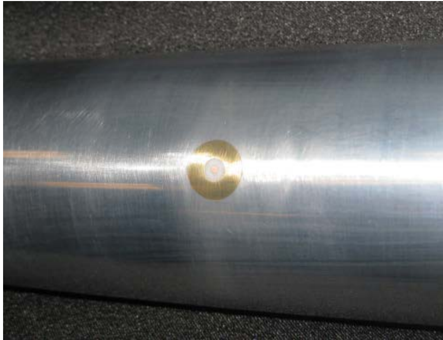
Fig. 4.29. Close up picture of glow perturber inserted in the cone-ogive-cylinder model for testing in the BAM6QT.
