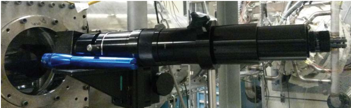
Fig. 4.21. Picture of the long-distance microscope used to measure the distance between the hot-wire probe and the surface of the cone-ogive-cylinder.
