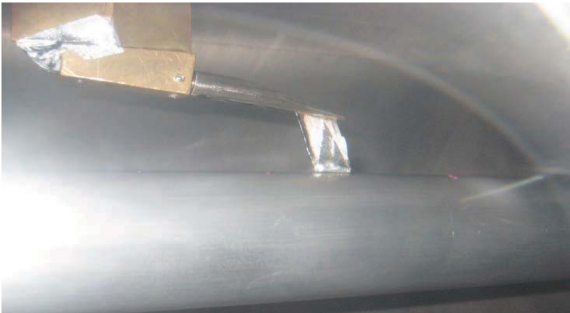
Fig. 4.19. Picture of the hot-wire probe installed inside the BAM6QT and held directly over the surface of the cone-ogive-cylinder.
