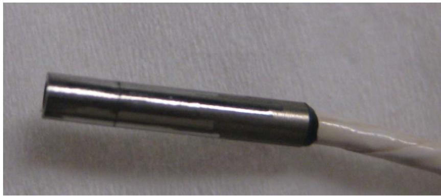
Fig. 4.15. Picture of a Kulite XCQ-062-15A pressure transducer.
