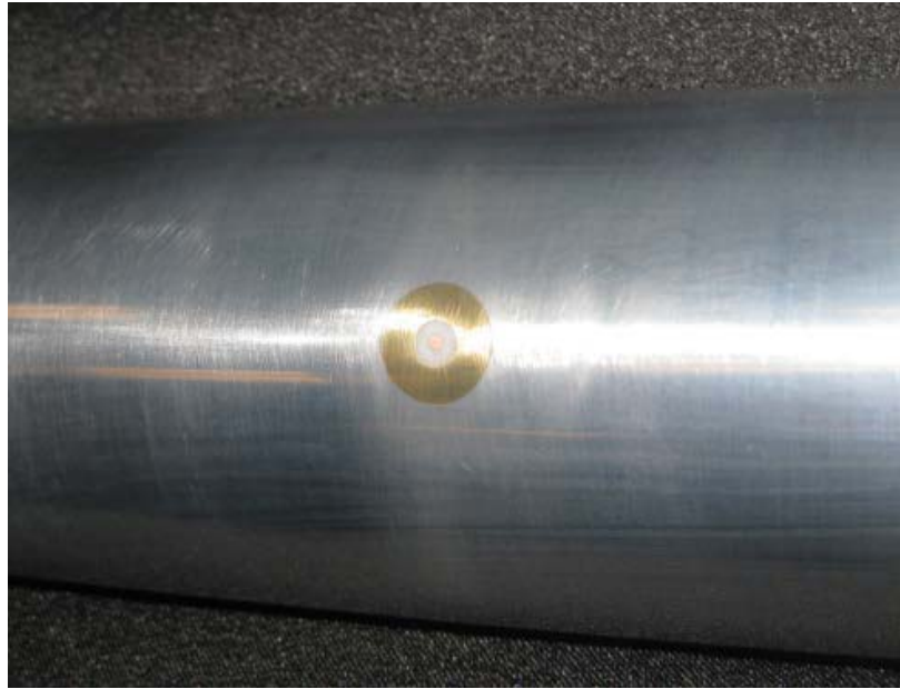
Fig. 6.16. Picture of the glow perturber electrodes installed flush on the surface of the cone-ogive-cylinder.
