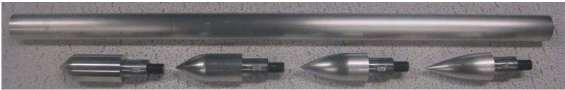
Fig. 4.5. Photo of cone-ogive-cylinder with interchangeable cone-ogive sections
