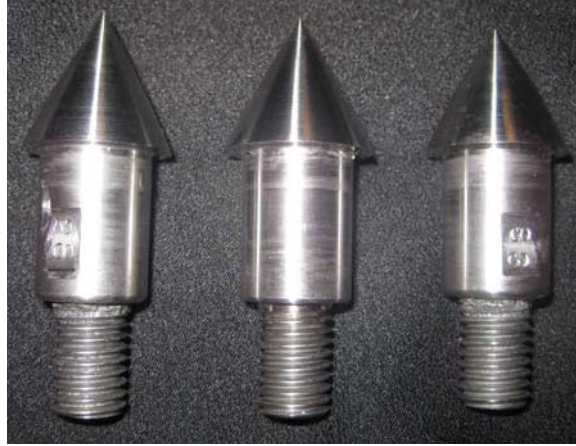
Fig. 4.3. Photo of 28, 30, and 33-degree nosetips for the cone-ogive-cylinder
