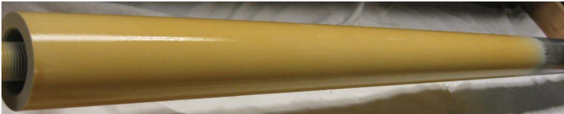
Fig. 4.14. Picture of the aft end of the cone-ogive-cylinder after being painted with TSP.
