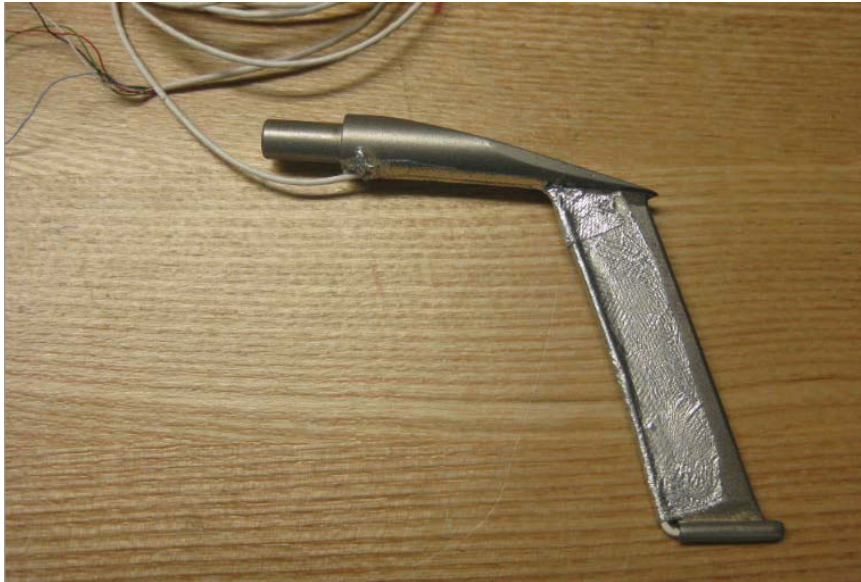
Fig. 4.16. Pitot probe with installed B-screen Kulite pressure transducer.
