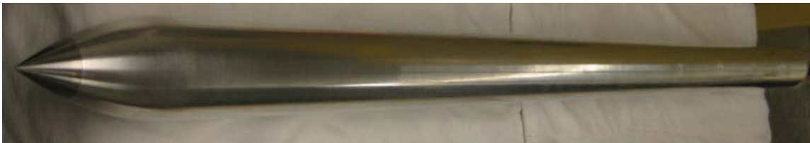
Fig. 4.2. Picture of the original cone-ogive-cylinder tested in the BAM6QT.
