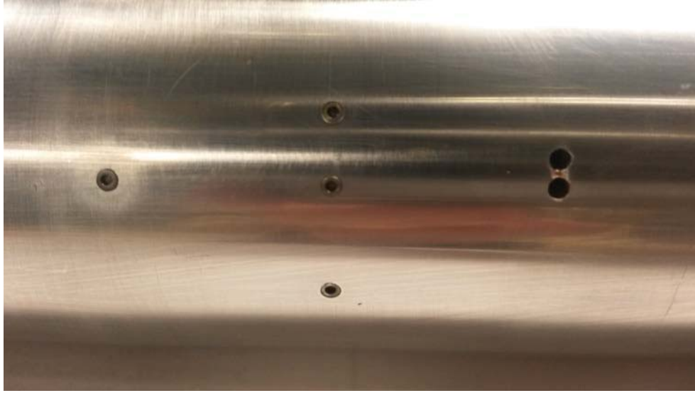
Fig. 4.10. Picture of Kulite pressure transducers at x=52 and 54 cm as well as two open sensor ports at x=56 cm.
