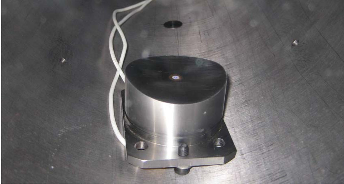
Fig. 4.31. Picture of the tunnel-insert glow perturber operating inside the Purdue vacuum test cell.
