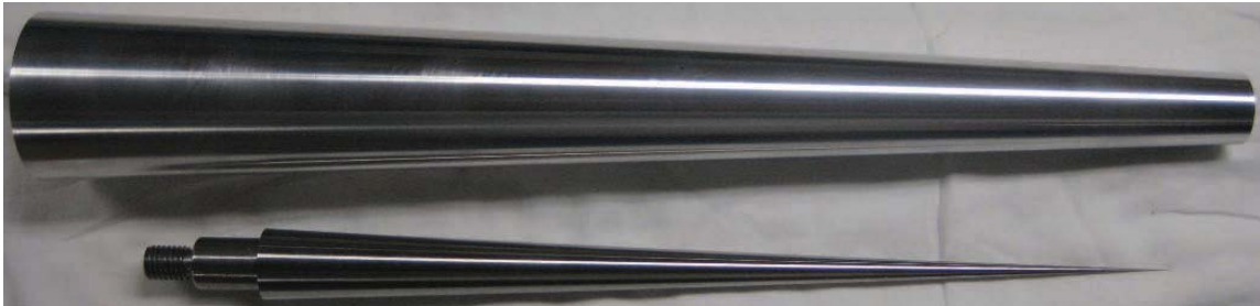
Fig. 4.12. Picture of the flared cone tested in the BAM6QT.
