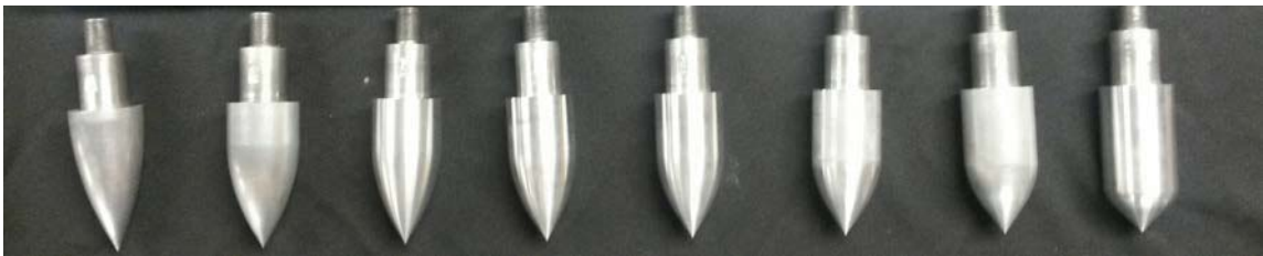
Fig. 4.7. Picture of all eight interchangeable cone-ogive portions of the cone-ogive-cylinder model.
