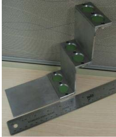
Figure 8: An image of the stair step sample fixture, with substrates loaded is shown.
