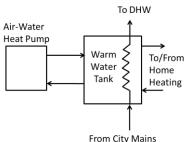
Figure 1: Air-Water Heat Pump Integration
