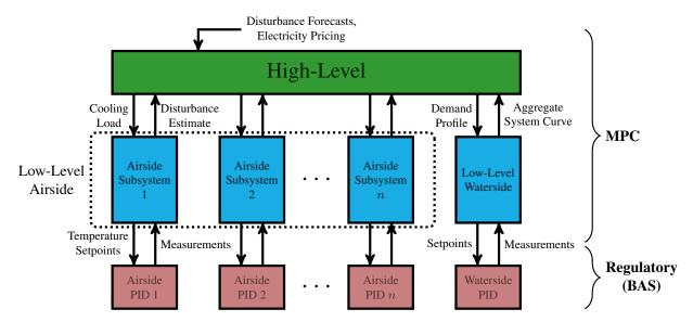
Figure 2: Control architecture with distributed MPC on the low-level airside problem (dotted box) for large-scale applications.
