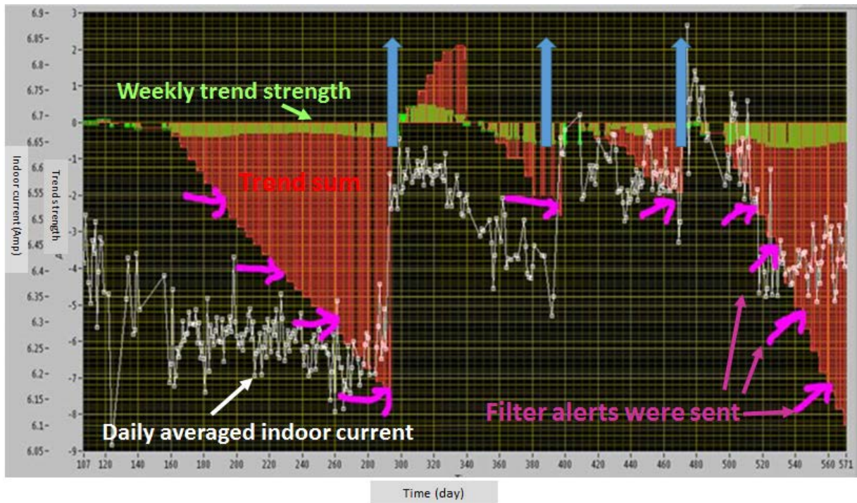
Figure 6: Results for the application of the Mann-Kindle algorithm over the daily averaged indoor current of a HVAC system for more than a year
