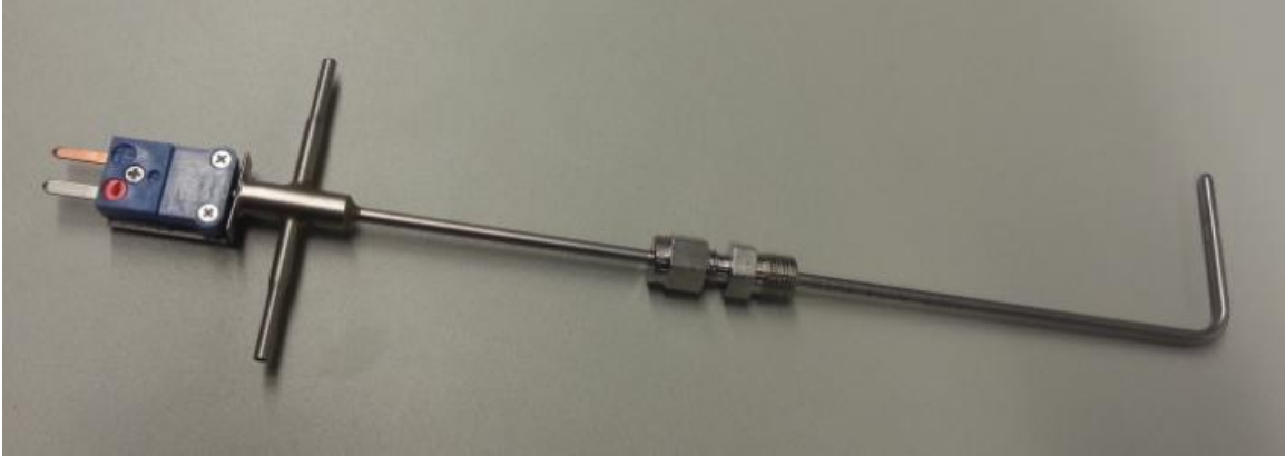
Figure 3.6: United Sensor PAC-T-8-K-KL-Mini plug pitot probe.
