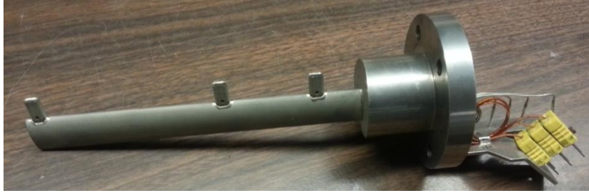
Figure 3.7: Three element inlet plenum total temperature and total pressure rake.
