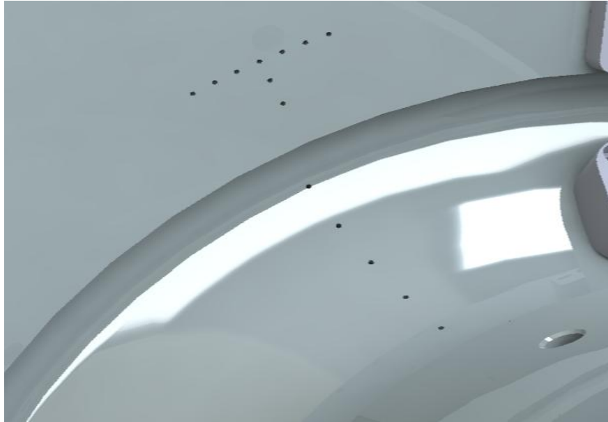
Figure 3.12: Impeller static pressure taps.
