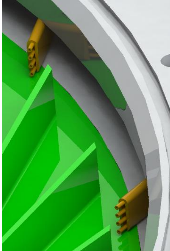
Figure 3.16: Two of the eight diffuser exit total pressure rakes.
