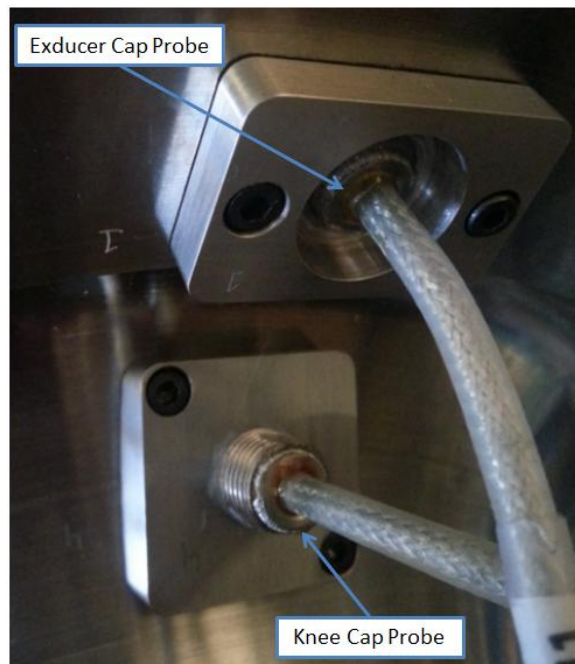
Figure 3.13: Knee and exducer capacitance probes used to measure blade tip clearance.
