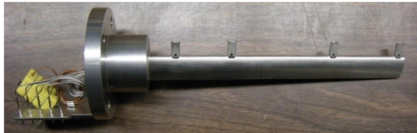
Figure 3.8: Four element inlet plenum total temperature and total pressure rake, from [27].
