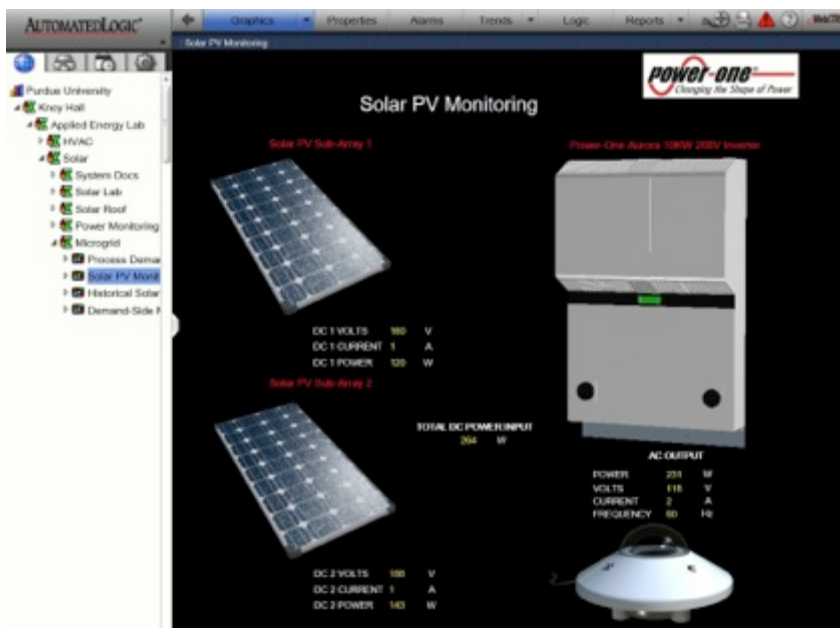
Figure 3.4 WebCTRL Graphic View of Solar PV Monitoring
