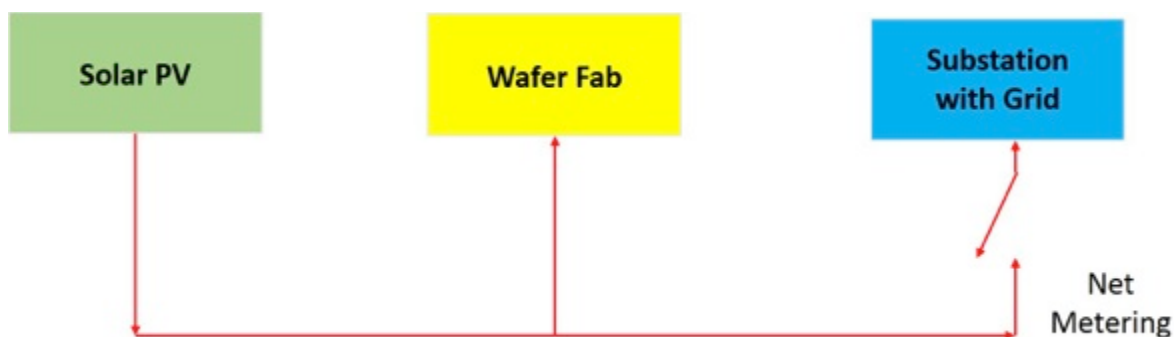
Figure 2.4 Schematic of Solar PV with Grid Integration, (Taboada et al., 2012)
