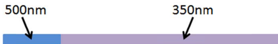
Figure 4.1 Capillary packed with 500 nm particles in the front, and followed with 350 nm particles.
