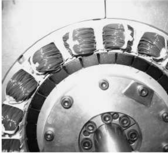
Fig. 1.10. Close up view of 6kW 36-slot/30-pole fractional-slot concentrated winding SM-PMSM used in [24]
