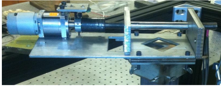
Figure 3-15: Variable impedance exit area developed by 463. The two plates form an exit opening that is varied by moving the plates relative to each other.
