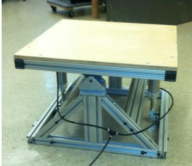
Figure 2-4: Second iteration balance board design shown with the low-friction pivots put in place within the system.
