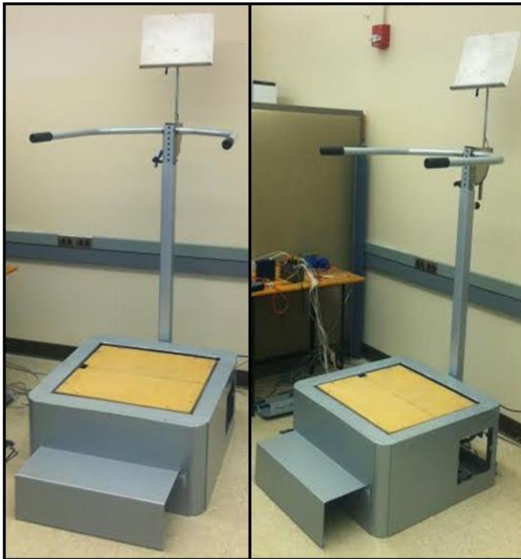
Figure 2-8: Final balance board shown along with the surrounding safety platform. A step was incorporated to simplify stepping onto the board, hand rails were manufactured to be adjustable to different heights, and access holes are placed in the base for easy access to hardware.
