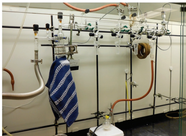
Figure 1. MBraun glovebox filled with inert N 2 atmosphere (left) and Schlenk line for air- and moisture-sensitive manipulations (right).
