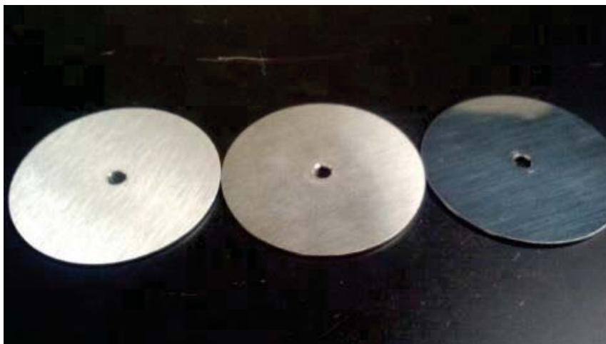
Figure 5.11. Wall friction test coupons used to measure friction coefficients (from left to right 1.20, 0.28, and 0.05 \mu\text{m} roughness).
