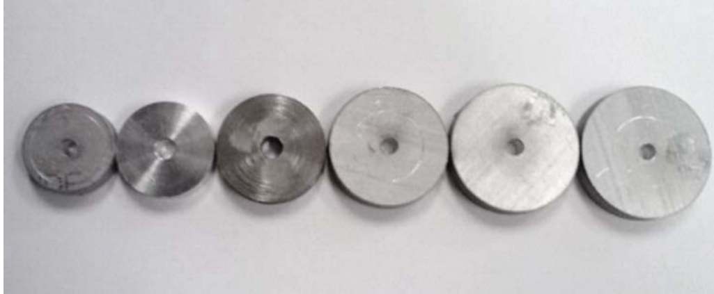
Figure 6.5. Image showing the plug attachments. The plug diameters from left to right are 2.09, 2.29, 2.50, 2.67, 2.85, and 3.04.
