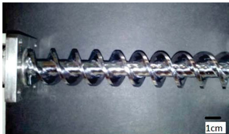
Figure 5.1. An image of the standard WP 120 Alexanderwerks Roll Compactor feed screw used in the experimental trials.
