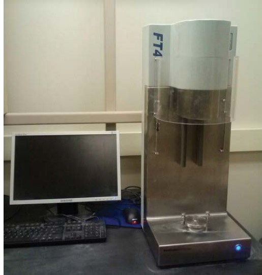
Figure 5.4. FT4 powder rheometer used for material characterization.
