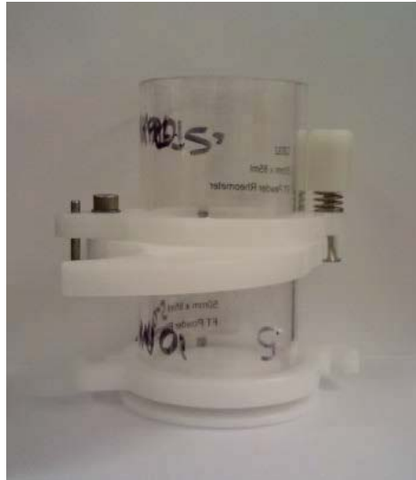
Figure 5.5. FT4 vessel for material testing.
