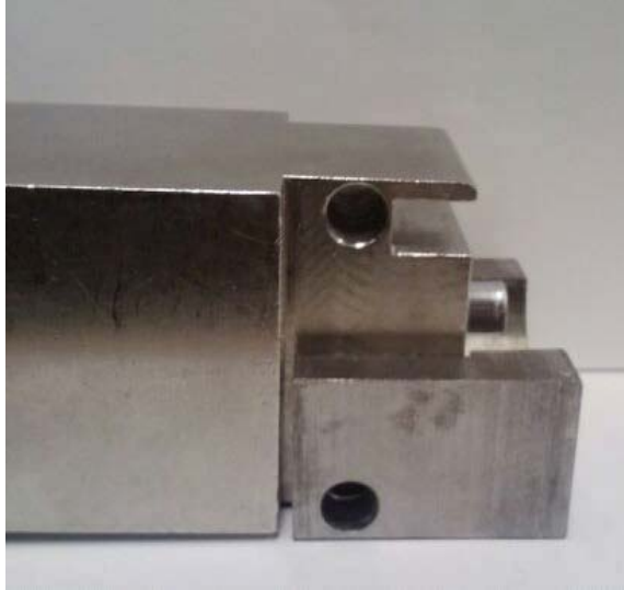
Figure 6.7. Image showing the feeder attachment (bottom) and the original feeder geometry (top).
