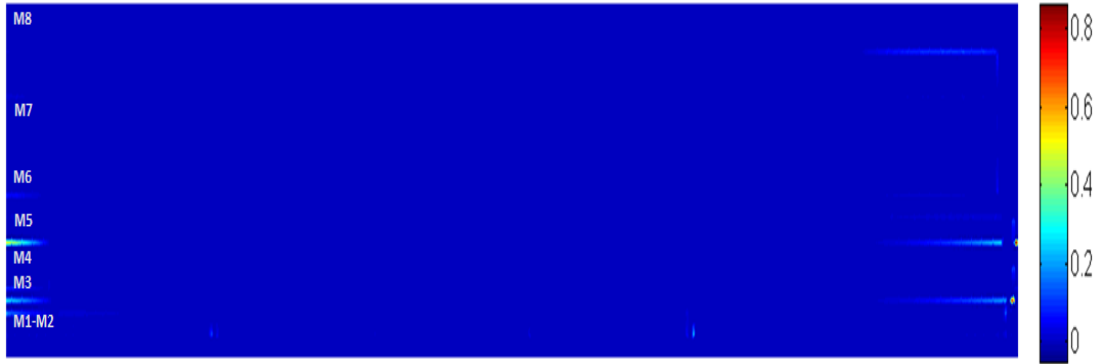
Figure 7-10. Damage accumulated during second peak excitation of ultrasonic stage, t=7.5 \text{ E-7 s} .
