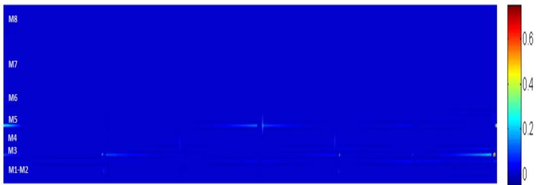
Figure 7-9. Damage accumulated during first peak excitation of ultrasonic stage, t=2.5 \text{ E-7 s} .
