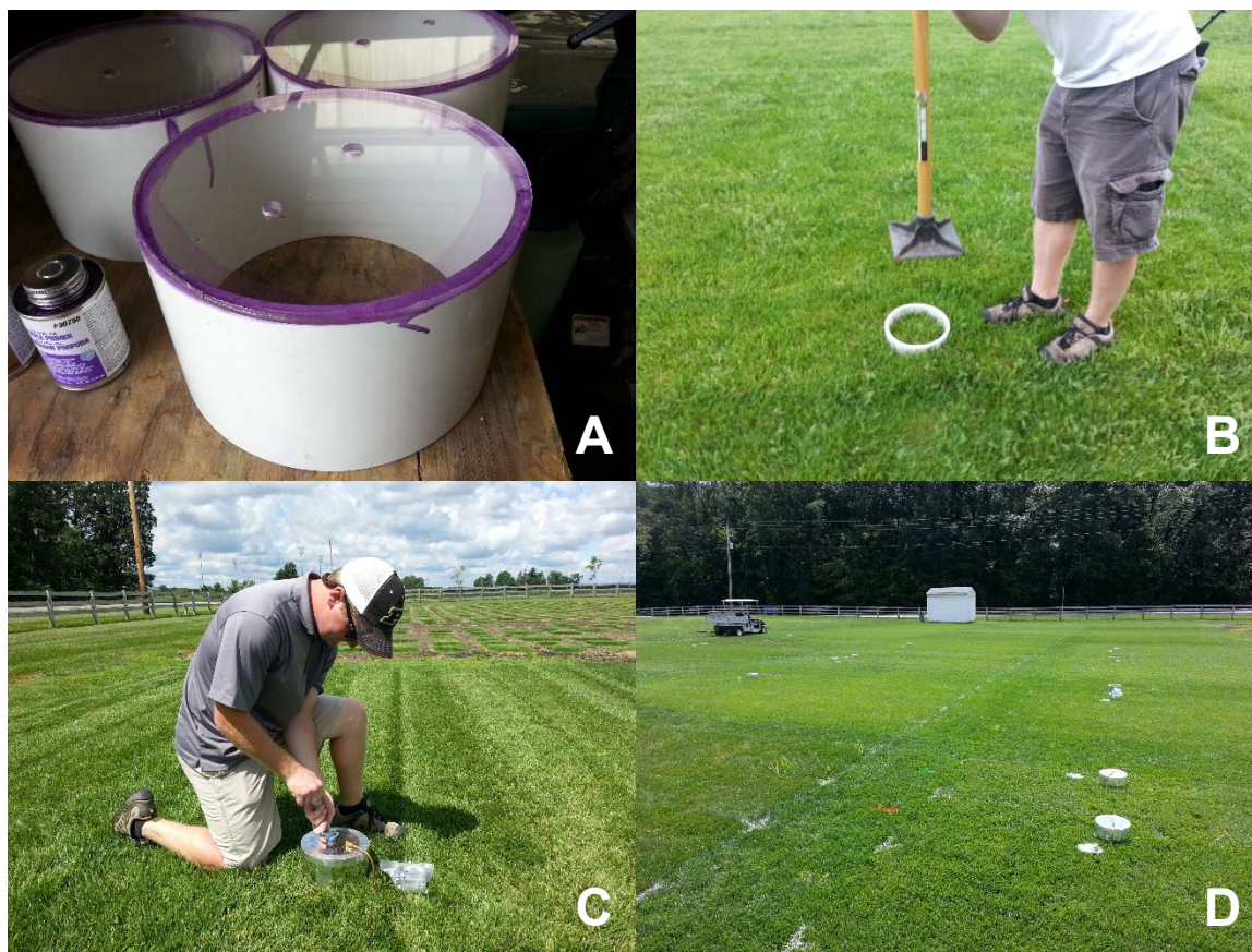
Fig. 4.1. Photos of the vented chamber construction (A), anchor installation (B), greenhouse gas sampling (C), and the experimental area with chambers installed (D).
