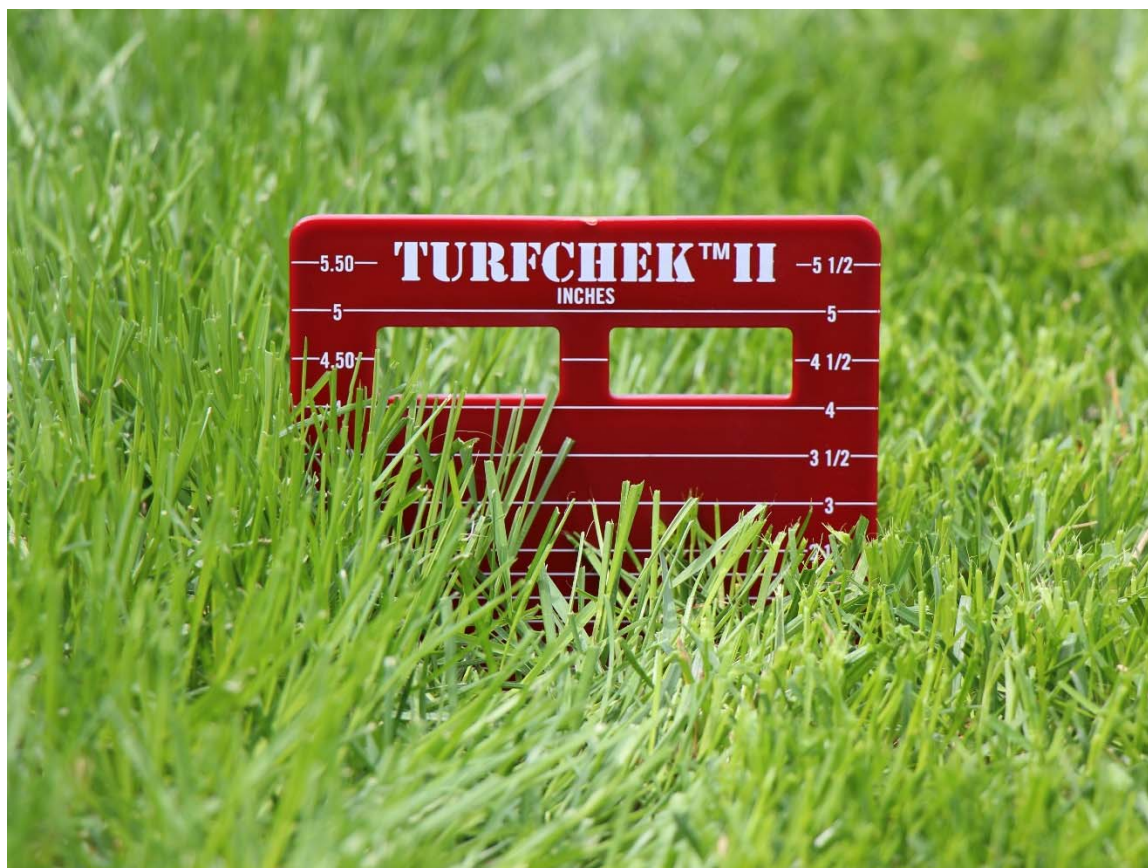
Fig. 2.1. TurfChek II grass height gauge (Turf-Tec International, Tallahassee, FL) used in this experiment.
