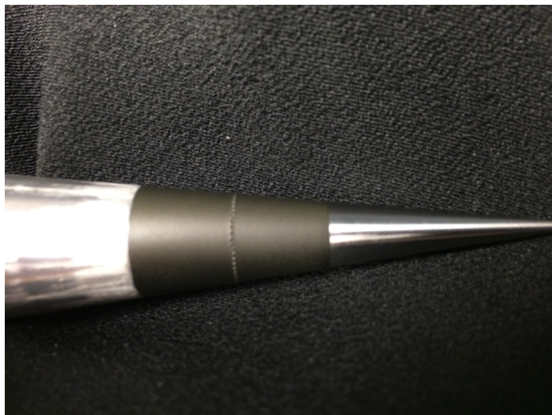
Figure 9.13. Photograph of Torlon insert assembled to the Ward Cone and nosetip.
