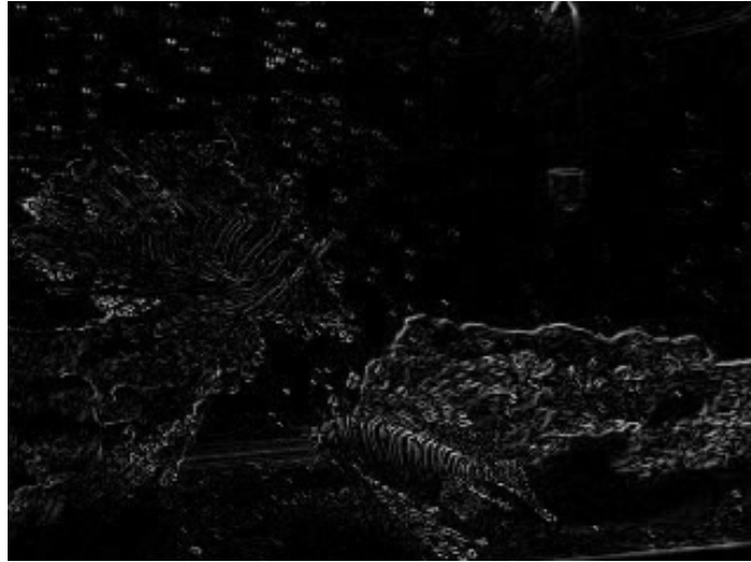
Figure 4.4: The absolute difference between two subsequent frames.
