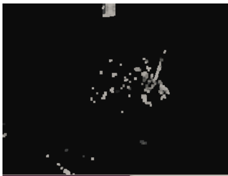
Figure 4.21: Back Projection Map After Dilation and Erosion.
