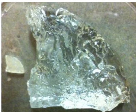
Figure 1. Synthesized poly(sodium acrylate-acrylamide) (PANa-PAM) with 67 wt.% PANa concentration and 2 wt.% crosslinking density in dry and swollen state (in deionized water for 2 days).
