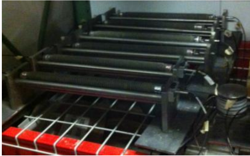
Figure 5. Sealed corrugated tubes filled with mortar mixture for autogenous strain test.
