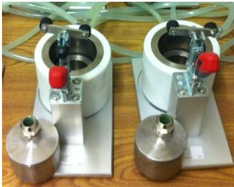
Figure 6. Rotronic chambers for relative humidity tests.
