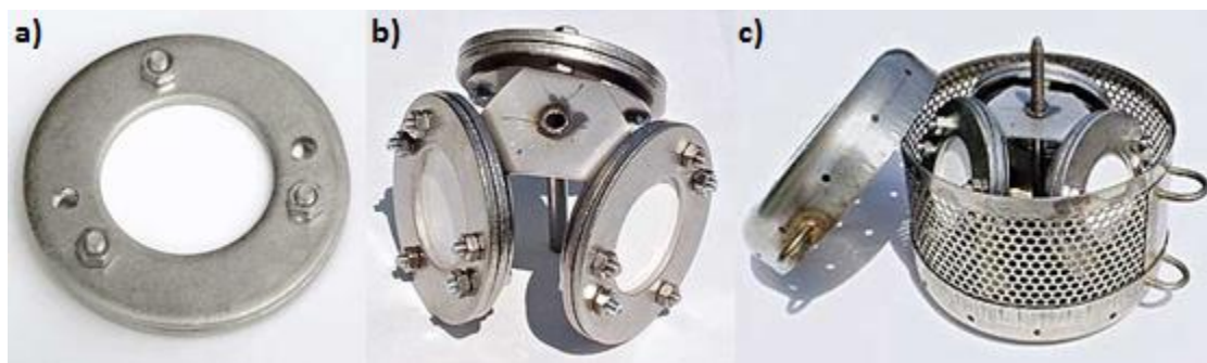
Figure 2.4 Polar Organic Chemical Integrative Sampler (POCIS): a) POCIS membrane, b) POCIS carrier, and c) POCIS holder.
