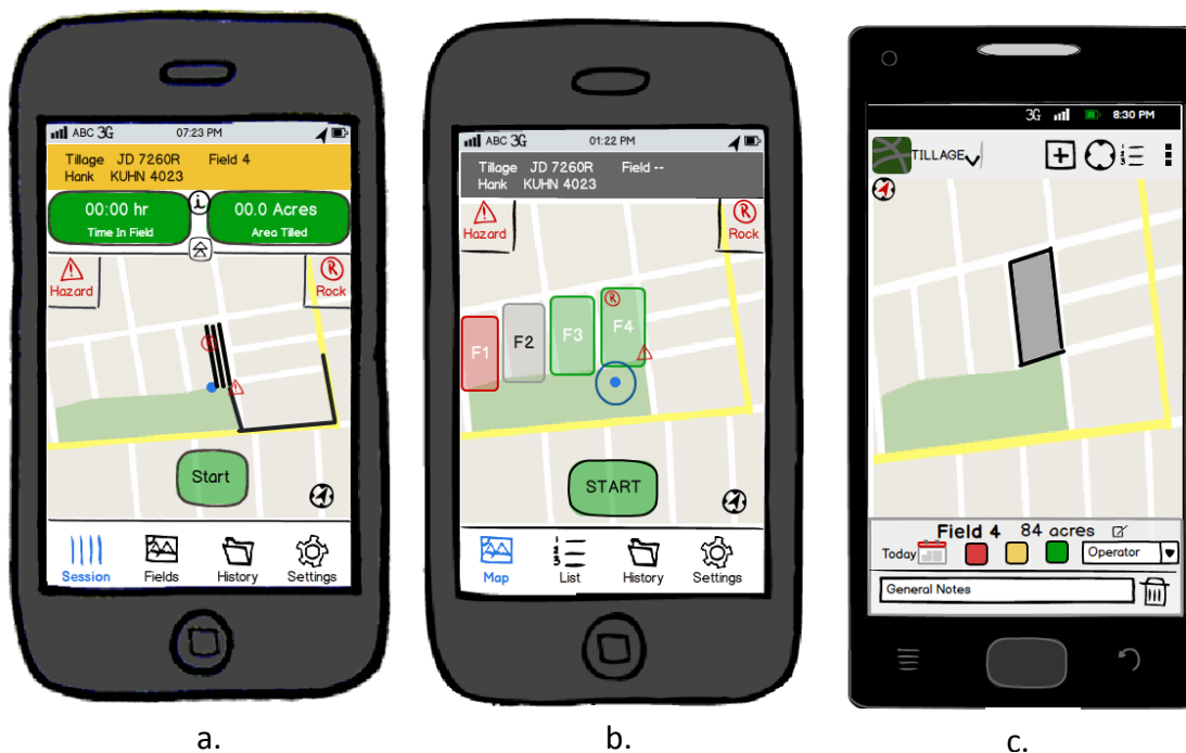
Figure 11: The progression of the Open ATK Tillage App mockups. (a.) The first mockup (Fall 2012) is a very function-heavy, user-tracking UI with Apple iOS themes. (b.) The middle mockup (Fall 2012) retained the Apple iOS themes but instead focused on the field operation status of each field. (c.) The last mockup (Spring 2013) adopted Android OS themes and a simplified UI, but retained the focus on the mapped fields.
