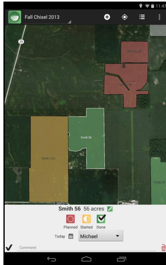
Figure 27: Screenshot of the Tillage App UI (V1.3) in a typical use scenario. The 56 acre Smith 56 field is selected and the menu allows the operator to record the date the operation was completed, his/her name, and any comments about the operation.
