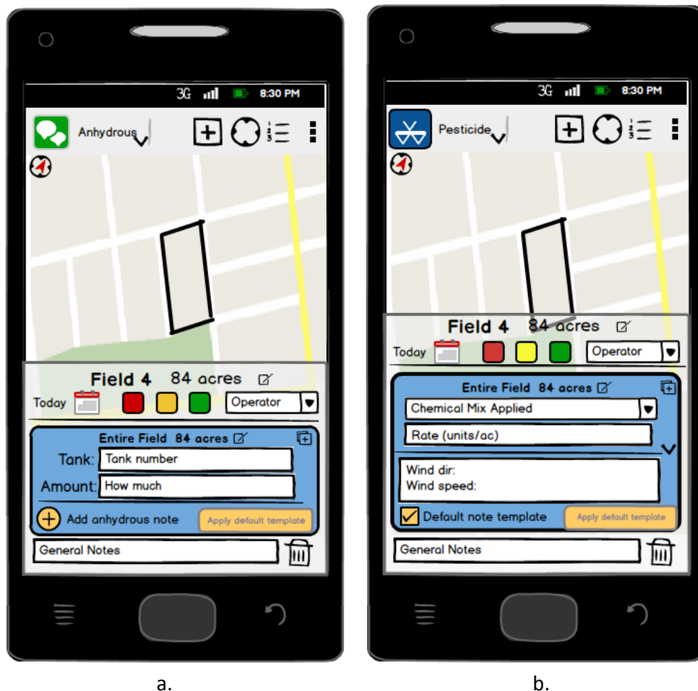
Figure 37: Early mockups of the OpenATK (a.) Anhydrous App and (b.) Spray App used to help farmers keep better records of field operations. Many UI components are reused for a consistent user experience and instant familiarity.
