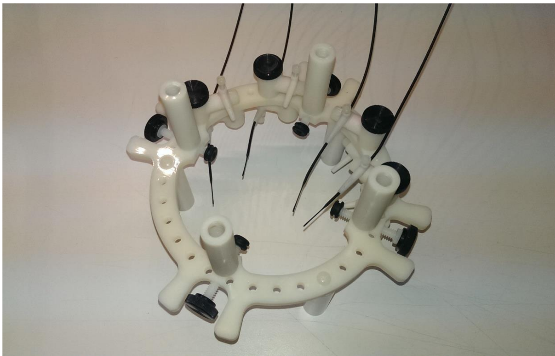
Figure 3.9 Test Fixture with Four Luxtron Probes used with Gradient Test Station
