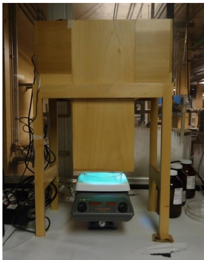
Figure 9. Collimated beam set-up at the Belmont WWTP Field Laboratory.
