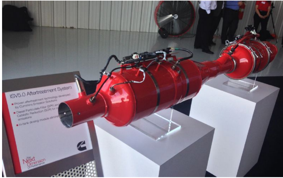
Figure 1.3. Aftertreatment System Used with a Cummins ISV Engine.
