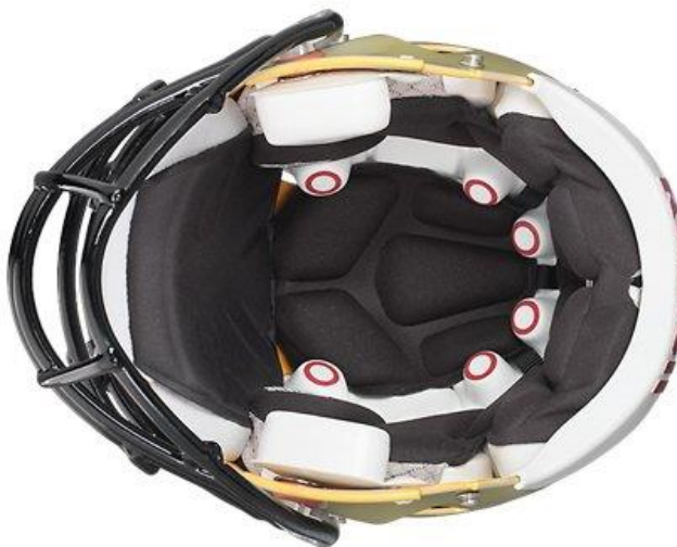
Figure 2.2. Riddell helmet fitted with a HIT system pod (white band with red, circular markings).
