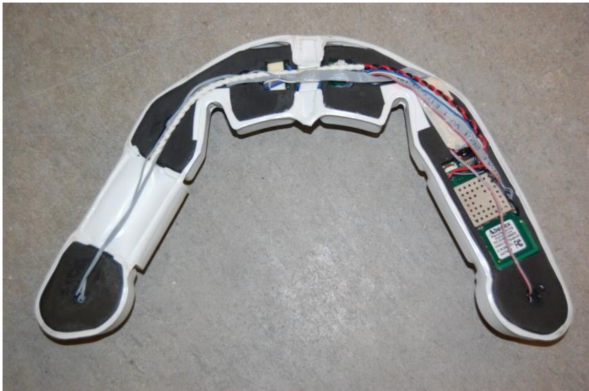
Figure 2.4. HIT System pod cutaway
