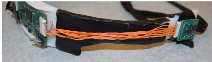
Figure 3.5. View of connectors and wiring harness
