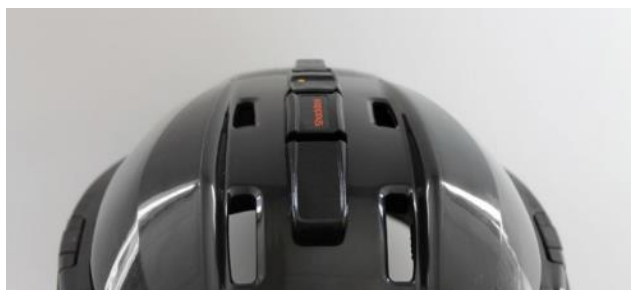
Figure 2.10. The Shockbox device mounted on a hockey helmet
