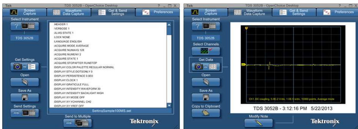
Figure 4.3 Tektronix OpenChoice Desktop Software is used to send settings and acquire data.
