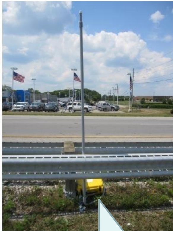
Short Term Battery Powered Device (Traffax)..Data post processed
