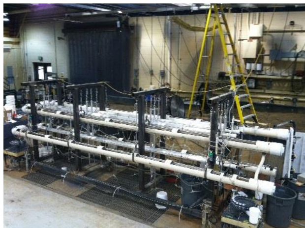
Figure 1. 20-m flume used in the instantaneous injection study (Yoder, 2013).
