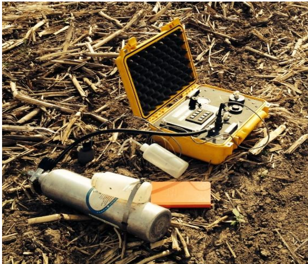
Figure 1. The cohesive strength meter (CSM).
