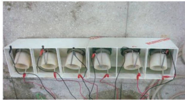
Figure 2. Tank of RCM equipment.
