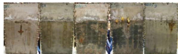
Figure 14. Mortar group ACC_M2 after acceleration test. #1 – OPC, equivalent 118 years; #2 – PC + 20%FA, equivalent 297 years; #3 – PC + 25%GGBS, equivalent 144 years; #4 – PC + 25%GGBS, equivalent 179 years; #5 – PC + 25%GGBS, equivalent 71 years.
