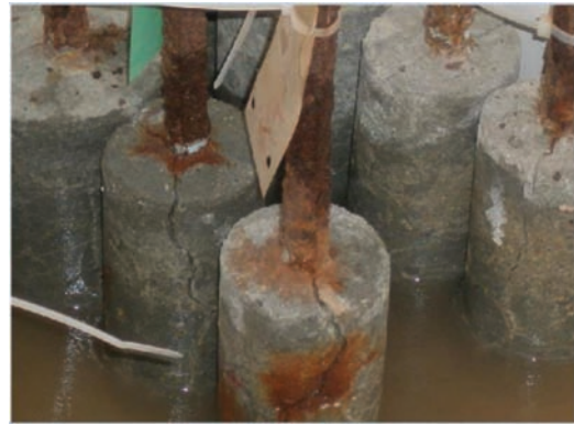
Figure 3. Sample of test-specimens exposed to chloride solution.
