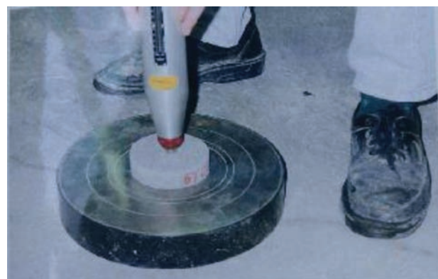
Figure 17. A setup of Rebound Hammer test.
