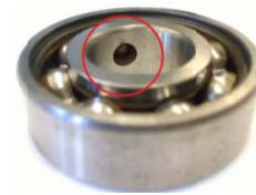
Fig. 9. Testing bearing with an inner-race fault.
