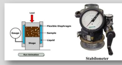
pressure devices. It tests the ability of the material to resist lateral spreading due to an applied vertical load.
