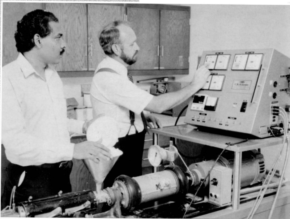
Starch-based bioplastic foam oozes from an extruder's nozzle as Rangan Chinnaswamy (left) adds starch and Milford Hanna adjusts controls. Using a process they invented, these IANR researchers produce extruded bioplastic foam made mostly of readily renewable and biodegradable materials. (Photo by Mark Hansen. Caption and photo courtesy RESEARCH Nebraska!)
