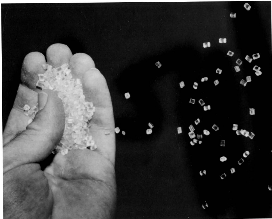
The extrusion process combines conventional plastic resin beads with starch, food chemicals and water to create functional, water-resistant, starch-based plastic foam containing only 20 percent polystyrene. (Photo by Mark Hansen. Caption and photo courtesy RESEARCH Nebraska!)
