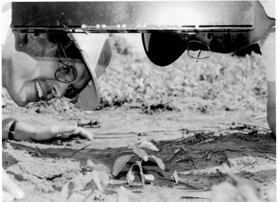
Weed Scientist Dave Mortensen (left) and Biological Systems Engineer Kenneth Von Barga calibrate the sensor on the weed sensor-intermittent sprayer system they're developing. This optical sensor distinguishes plants from soil background. (Photo by Mark Hansen. Caption and photo courtesy RESEARCH Nebraska!)
