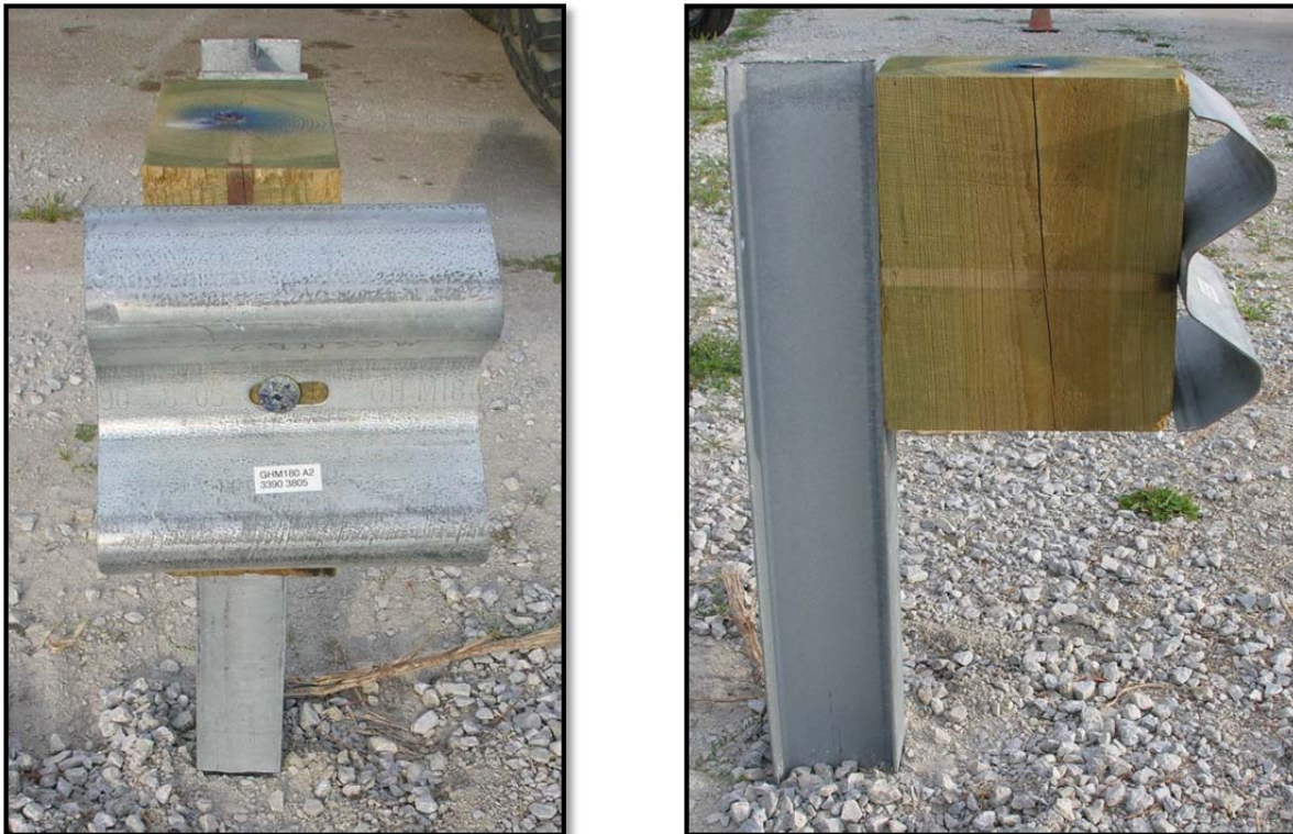
Figure 114. Test Setup to Measure Guardrail Bolt Torque
