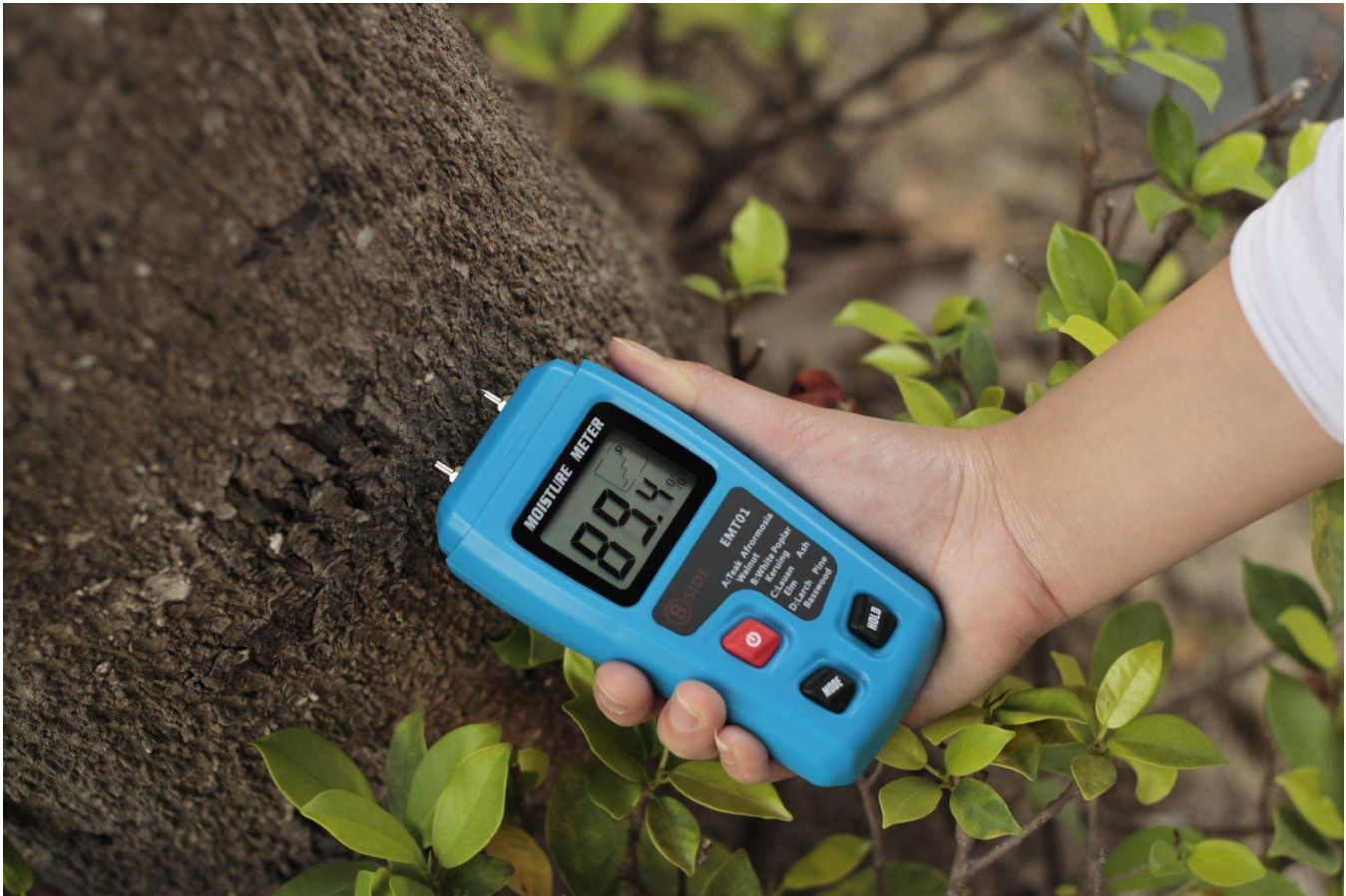
Figure 2.2 Electronic moister meters for timber
