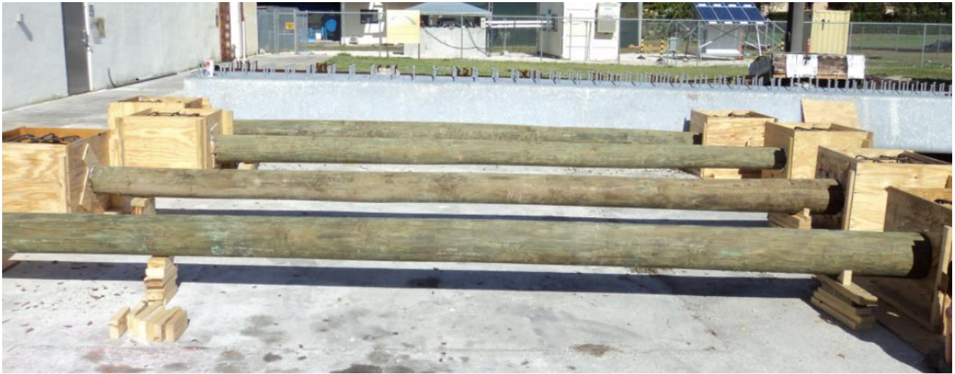
Figure 5.1: Full Scale timber pile test specimens
