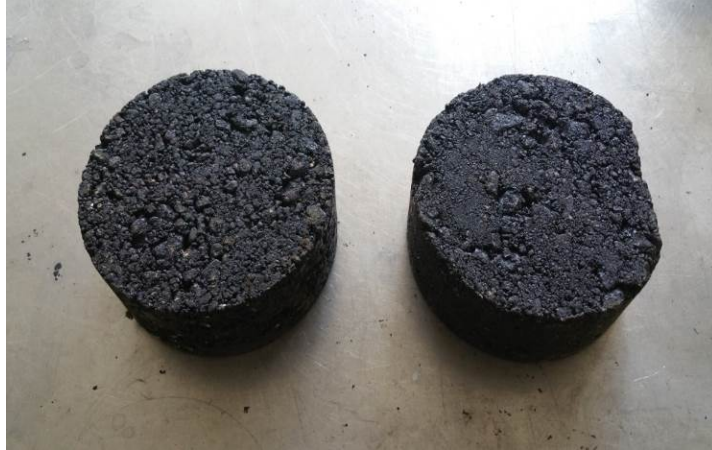
(a) cut specimen after compaction
