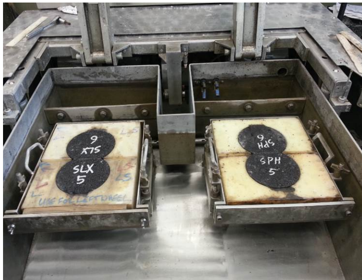
(b) cylindrical specimen mounting system
