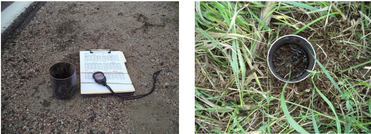
Figure 2-5. Measurement of initial water infiltration at the Beaver Crossing site.
