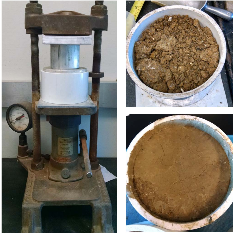
Figure 2-6. The hand-operated hydraulic press used to compact soils (left). Soil before and after compaction (right).
