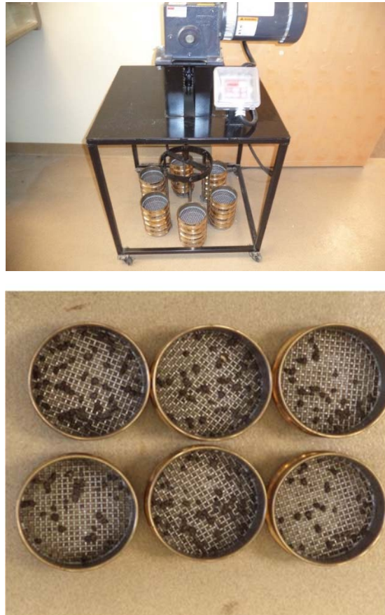
Figure 2-4. Mechanical sieving equipment (top) and sieves (bottom) used for the determination of wet soil aggregate stability in the laboratory.
