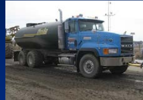
S5 (Homemade 4400 gal – flotation tires)
