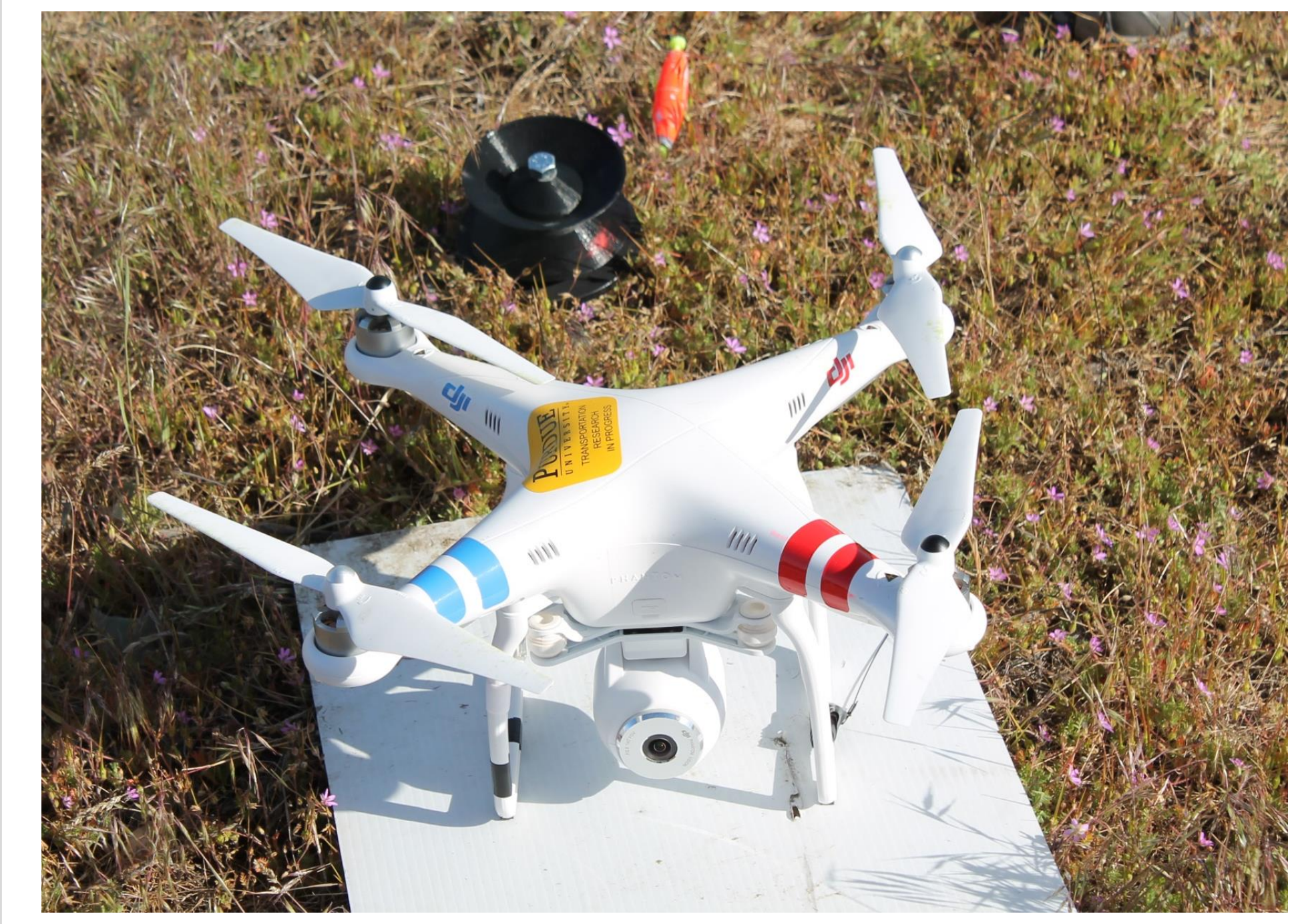
To observe the entire interchange, an aerial camera was used to record operations. The height advantage allowed the operations to be observed in a single frame. The drone was GPS-assisted and tethered while flown at an altitude less than 100'.
