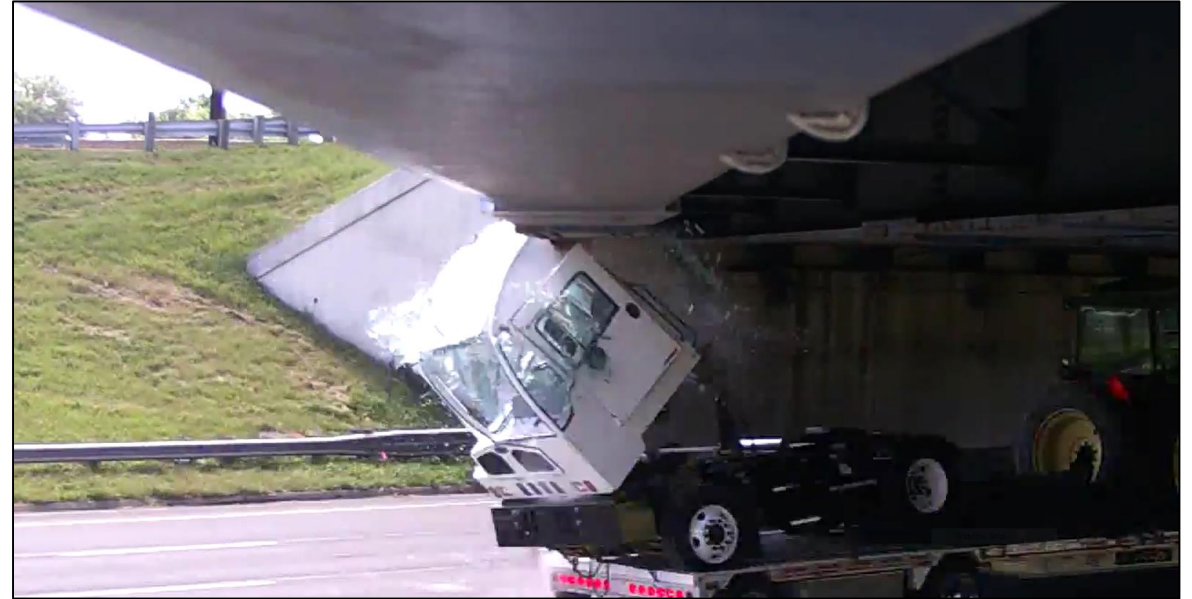
Example Bridge Strike on NB I-65/I-70 “South Split” Corridor
